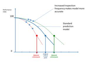
An alternative approach to aid existing degradation models is to perform frequent inspections to provide more data points relative to the actual degradation of the roadway. With its integrated maintenance and update workflow functions, RUBIX is an ideal tool for such an approach.
